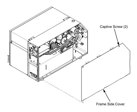
Figure 2. Removing the Frame Side Cover
